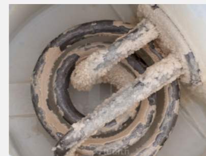
Example of lime-scale deposits from hard water areas.
